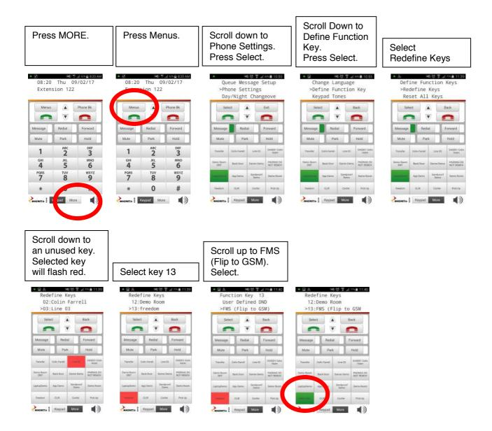
When you are on a call you now will have the option to flip between VoIP and GSM by pressing the function key which you have defined here.
